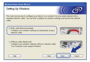
8 Connect the Brother wireless device to your access point using a network cable and click **Next**.
